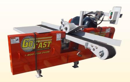
The Go Fast 6 x 8 Master Resaw is a universal and adaptable band resaw that is great for all sawing needs. The compact design and variable speeds allow it to fit into any operation. The 6 x 8 Master is resaw is accurate and easy to adjust. Multiple head configurations are available up to 6 heads.
